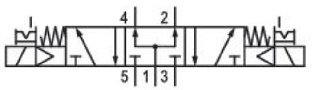
Industrial Electrically Spool valve, positive overlapping Pressurized Center Double Solenoid metal/metal sealing Plate connection
