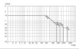
v<sub>t</sub> = Piston velocity [m/s] m = Cushionable mass [kg]
