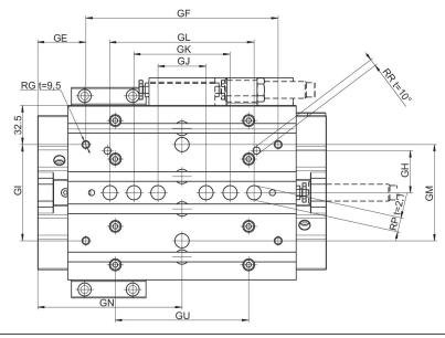
− t = depth \* CKP 16: 2x Lube ports on each runner block, CKP 25 / 30: Lube nipple of funnel type with thread connection M3
