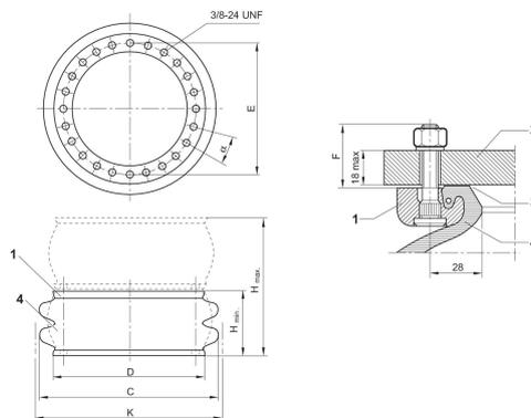
section of mounted bead ring with staybolt 1. mounting ring 2. machine part 3. sealing surface \*) 4. bellow \* recommendation for surface finish: if
