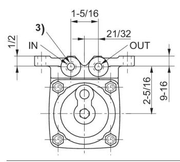
1) 0.031" eccentric screw for total roller adjustment of 0.062" to obtain 2.531" "A" dimension 2) Mounting hole Ø13/32 3) 1/4 - 18 NPTF
