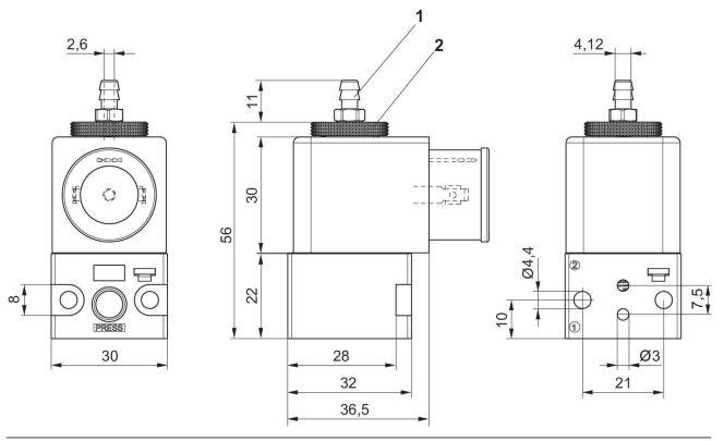
1) Tightening torque: 0.8 Nm ±0.01
