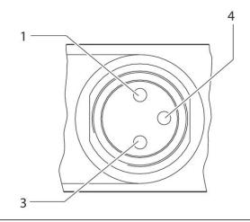
1) Pin not assigned 3) 0 V 4) 24 V Note: Bi-polar protective circuit to prevent overvoltage
