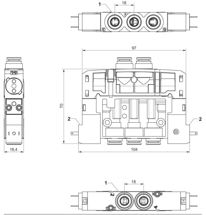
1) Connections [1,3,5,2,4] Ø 8 2) 2 pilot valves with external electrical connection
