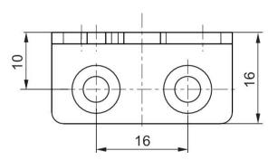
2 countersunk screws DIN 7991 A4 M4x8 for mounting on AV series pressure regulators are included in the scope of delivery. Countersunk screws for mounting on a mounting plate are not included in the scope of delivery.
