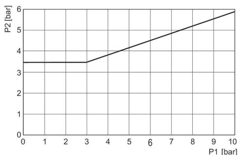
p1 = pression aux raccords 2 et 4 , p2 = pression de pilotage
