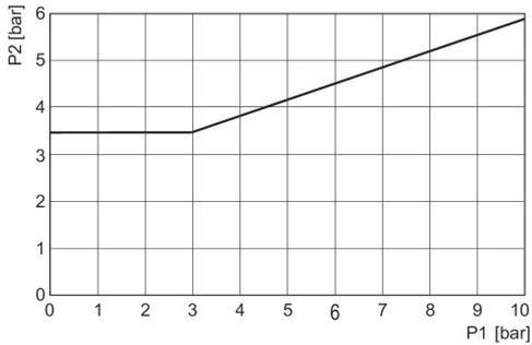
p1 = pressure on connections 2 and 4, p2 = control pressure
