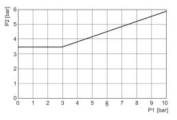
p1 = pressure on connections 2 and 4, p2 = control pressure
