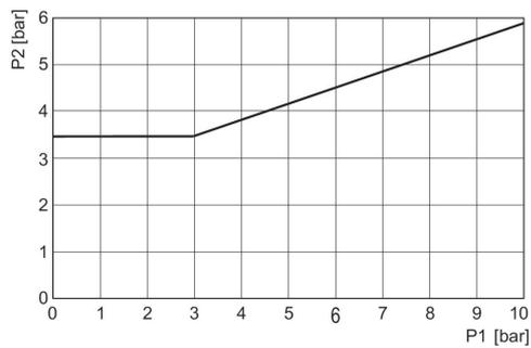
p1 = pression aux raccords 2 et 4 , p2 = pression de pilotage
