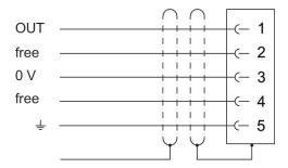
Sensor round plug M12x1, 5-pin, integrated socket, A-coded The ground for plug X20 PIN 5 and the shielding for plugs X7E1 / X7E2 and X20 are directly connected to the housing. The device must be mounted on a grounded mounting plate.
