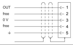
Sensor round plug M12x1, 5-pin, integrated socket, A-coded
