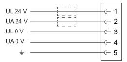
Sensor round plug M12x1, 5-pin, integrated plug, A-coded Only use a power pack with safe isolation for power supply (electronics and actuator power).
