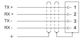
Ethernet plug M12x1, 4-pin, socket, D-coded The Ethernet cables must be shielded.
