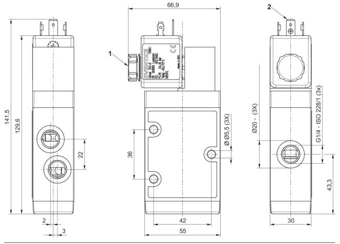
1) Silencer 2) Valve plug connector form A, EN 175301-803
