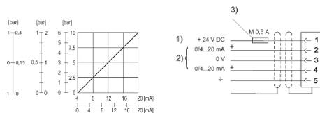
1) Supply Voltage 2) Actual value (pin 4) and nominal value (pin 2) are related to 0 V. Current control (ohmic load 100 Ω). Actual value output (max. total resistance of downstream devices < 500 Ω). 3) The operating voltage must be protected by an external M 0.5 A fuse. Connect the plug via a shielded cable to ensure EMC.
