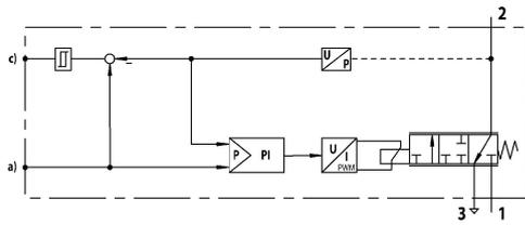
a) Nominal input value c) Switch output (acknowledge signal) The E/P pressure control valve modulates the pressure corresponding to an analog electrical nominal input value.
