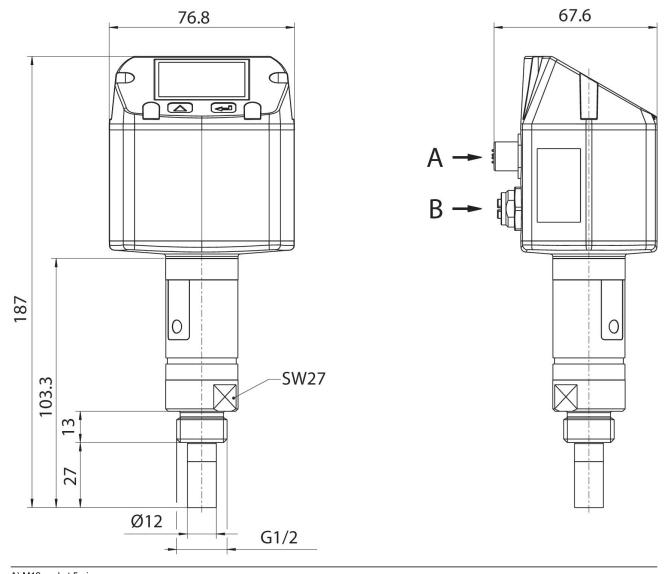
A) M12 socket 5-pin B) M12 socket, 8-pin
