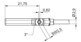
1\* = switching point 2\* = locking screw 3\* = LED window, transparent L = cable length
