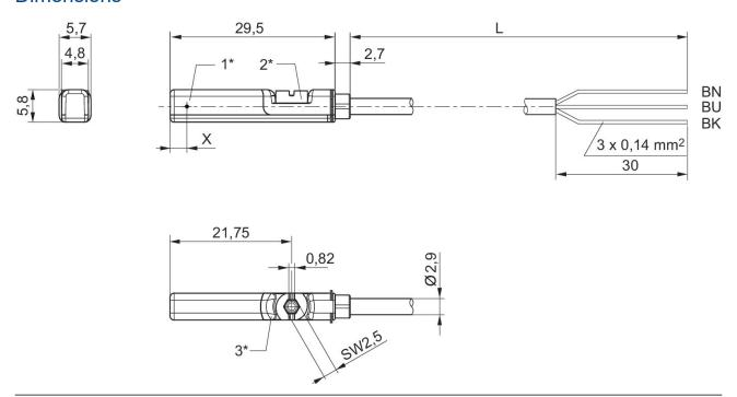
$<sup>1^*</sup>$  = switching point  $2^*$  = locking screw  $3^*$  = LED window, transparent L = cable length BN = brown, BK = black, BU = blue X = electronic: 11.6 mm
