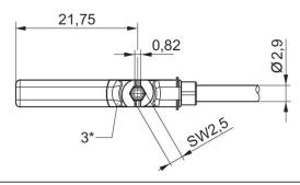
$<sup>1^*</sup>$  = switching point  $2^*$  = locking screw  $3^*$  = LED window, transparent L = cable length BN = brown, BK = black, BU = blue X = electronic: 11.6 mm
