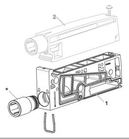
material: housing: Polyamide, fiber-glass reinforced \* For more information on push-in fittings, see the "Push-in fittings" page for the AV series in the catalog.
