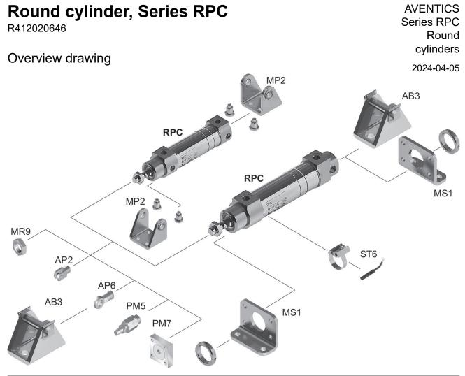
NOTE: This overview drawing is only for orientation to indicate where the various accessory parts can be fastened to the cylinder. The illustration has been simplified for this purpose. It is thus not possible to derive the dimensions from this overview.
