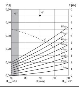
V = volume H = height H\* = recommended operating height for vibration isolation H\*\* = use permitted only upon approval by AVENTICS 1 kN = 1000 N
