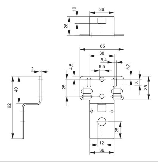
For assembly of the W01 mounting plate, the rear cover of the air preparation unit must be removed.
