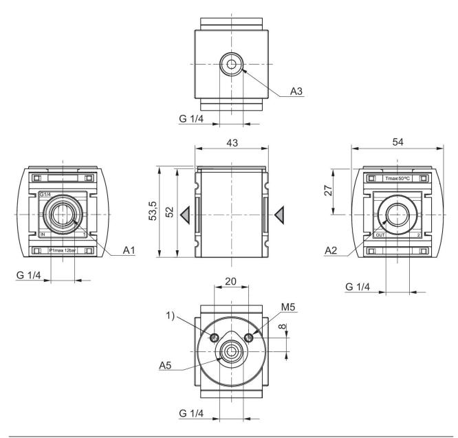
A1 = input A2 = output A3 = output A5 = output 1) Mounting thread for pressure sensor
