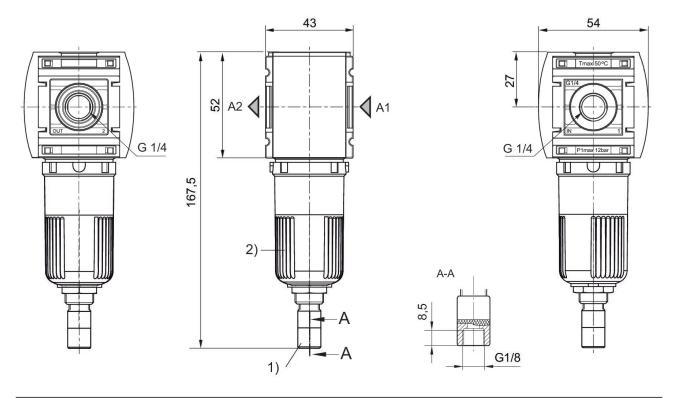
Fully automatic condensate drain
