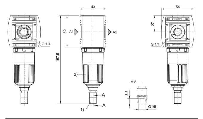
1) Fully automatic condensate drain 2) Reservoir: polycarbonate
