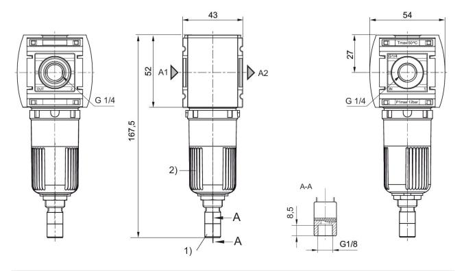
Fully automatic condensate drain
