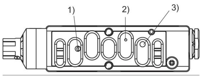
For use with a subbase with ISO 15407-1 hole pattern 1 = test pressure 2 = nozzle connection 3 = cleaning pressure
