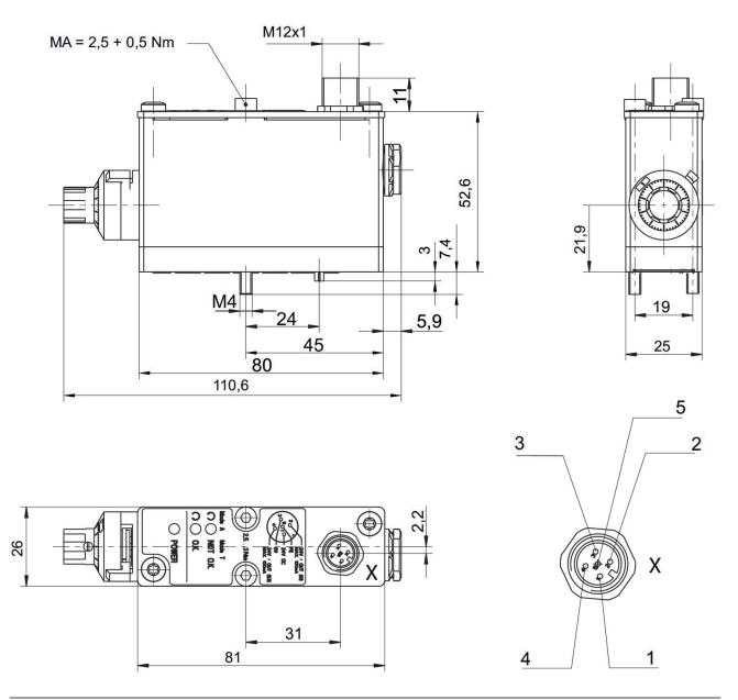
M12 contact assignment: contact 1: 24 V DC contact 2: output signal 24 V DC, S1 (working pressure), max. 100 mA contact 3: 0 V contact 4: output signal 24 V DC, S2 (testing), max. 100 mA contact 5: FE
