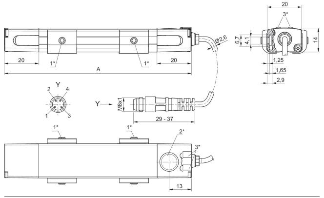
1\* = threaded pin M3x11 2\* = teach area 3\* = LED A = sensor length Pin assignment: 1 = (+), 2 = (OUT 1) 3 = (GND), 4 = (OUT 2/IO-Link), EN 60947-5-7 LED 1: yellow = measuring operation, red = error LED 2: green = voltage signal, blue = current signal
