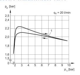
p1 = Working pressure p2 = Secondary pressure qn = Nominal flow
