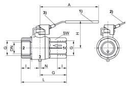
Note: Can only be locked when closed! Padlock not included in the scope of delivery.
