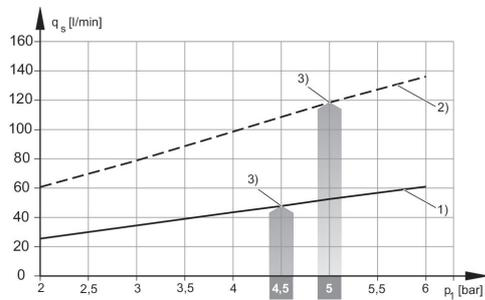
1) = Ø buse 1,0 mm 2) = Ø buse 1,5 mm
