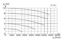
p1 = Working pressure p2 = Secondary pressure qn = Nominal flow
