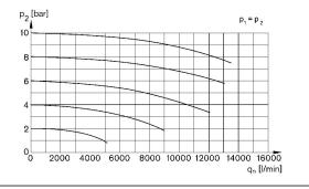
p1 = Working pressure p2 = Secondary pressure qn = Nominal flow
