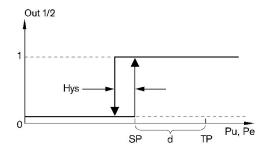
Vacuum sensor: d=20% Pressure sensor: d=5%
