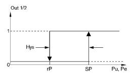
SP = switch-on point, rP = resetting point OUT: switch output
