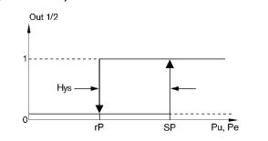
SP = switch-on point, rP = resetting point OUT: switch output
