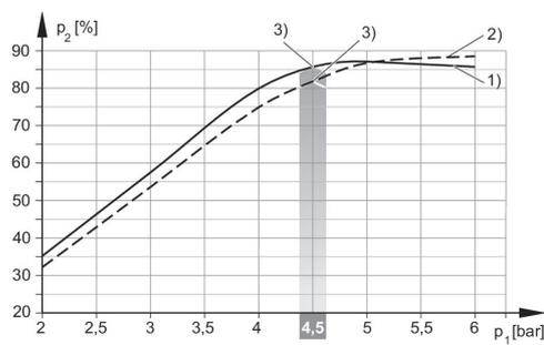
1) =  $\varnothing$  ugello 2,0 mm 2) =  $\varnothing$  ugello 2,5 mm
