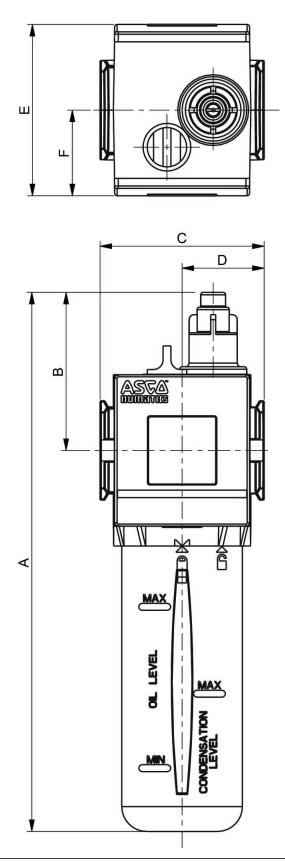
To remove the reservoir, allow a clearance of [[20] mm] from the bottom of the reservoir drain.
