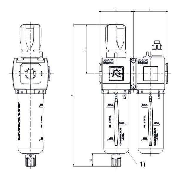
1) To remove the reservoir, allow a clearance of [[80] mm] from the bottom of the reservoir drain.
