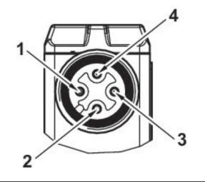
1) not assigned 2) Coil 12 3) 0 V DC 4) Coil 14
