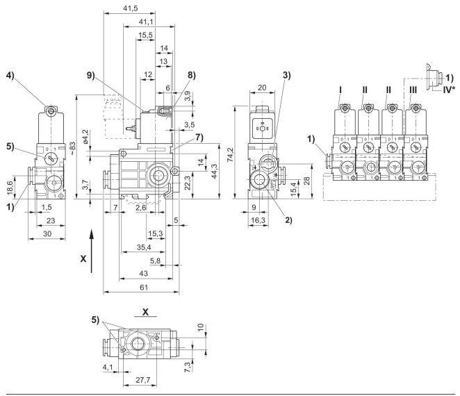
1) Port 1 2) Port 2 3) Port 3, exhaust air must not be throttled 4) Core Ø for M5 5) Manual override 6) Pocket hole 6 mm deep for 3.5 self-tapping screw 7) Mounting space for name plate 8) Coil can be rotated at 180° intervals 9) LED \* Air conn. module (item IV) mounted onto stacking valve (item II) permits additional air supply from right hand side. End valve (item III) not required. I = Inlet valve, II = Stacking valve, III = End valve
