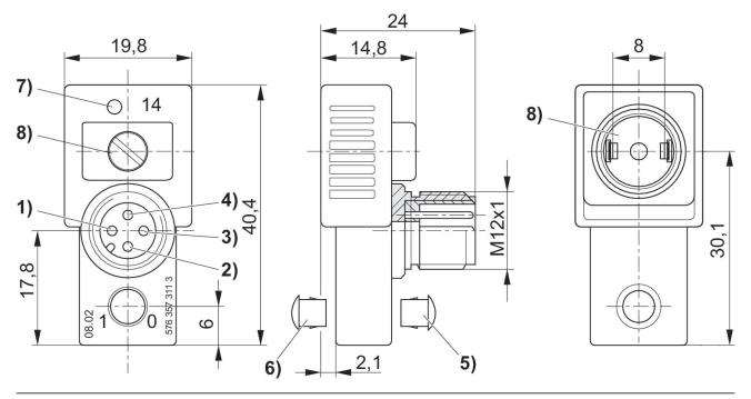
1) not assigned 2) not assigned 3) 0 V 4) magnet 14 5) Sealing cap for manual override not removable
