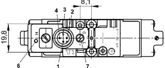
1) not assigned 2) not assigned 12 3) 0 V 4) magnet 14 5) metal round plug M12x1 6) yellow valve switching state LED 7) manual override
