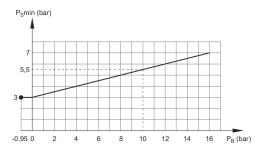
P<sub>B</sub> = Working pressure PS = control pressure
