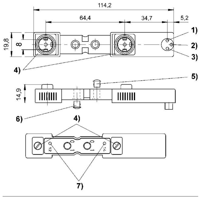
1) solenoid 14##2) solenoid 12##3) 0 V## 4) captive seal and screw##5) sealing cap for manual override not removable##6) removable##7) LED valve
