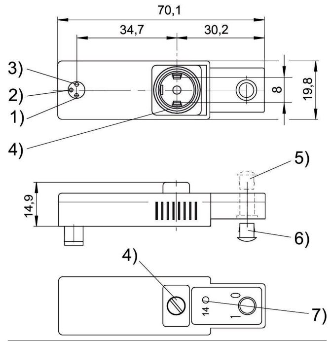
1) solenoid 14##2) not assigned##3) 0 V## 4) captive seal and screw##5) sealing cap for manual override not removable##6) removable##7) LED valve
