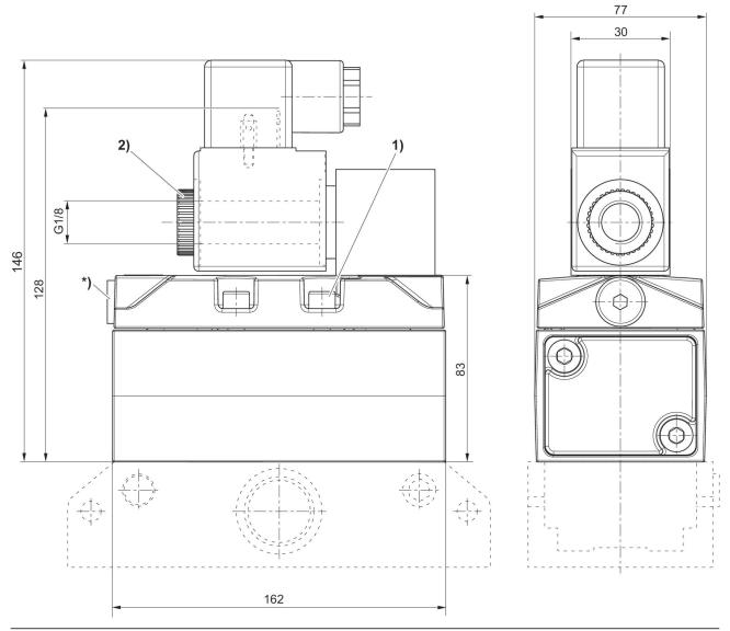
Tightening torque for mounting screws: 2.2 ± 0.2 Nm
