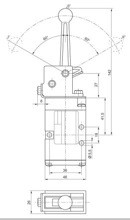
Position 0: initial position, position I: with detent, manual return, position II: automatic spring return.
